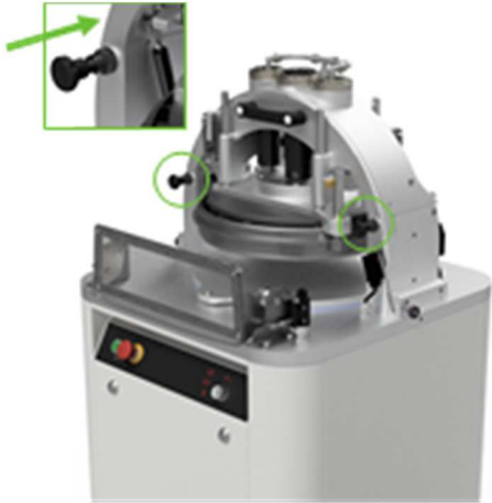
7. Close the fastening thrusters (x2)
