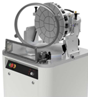
2. Remove the ring and clean it inside with a plastic scraper.
