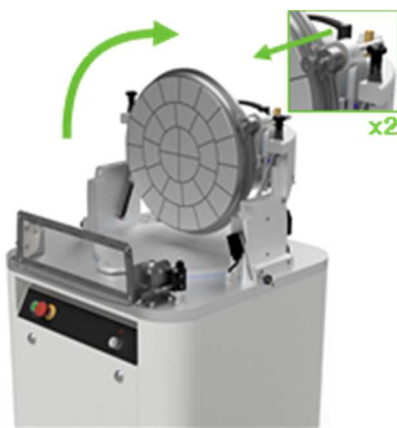
1. Open the cutting unit accompanying it to the support. Remove the ring fastenings (x2)
